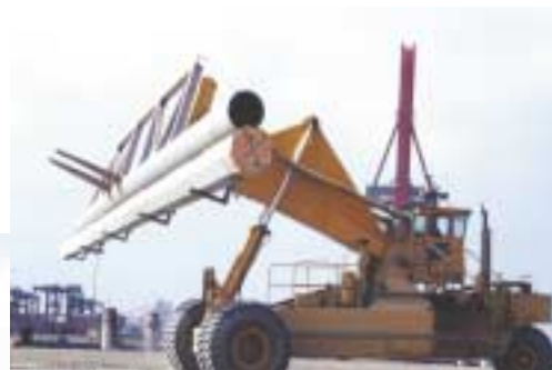
Handling and driving 30 ton concrete piles from shore.
