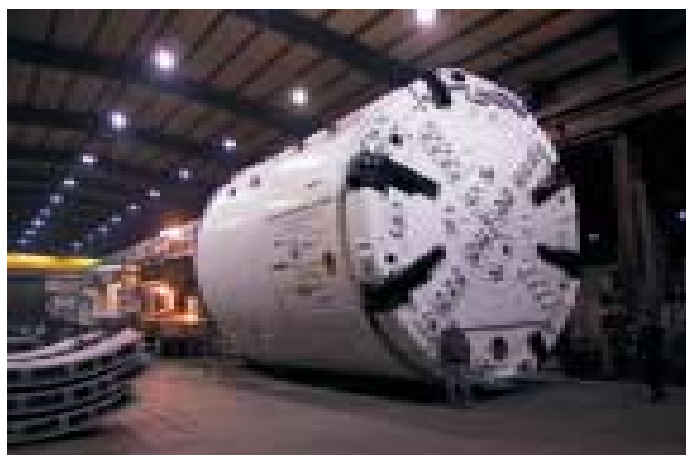
This fully-shielded TBM was designed to allow a bolted, gasketed segmental liner to be installed in the tail shield.
